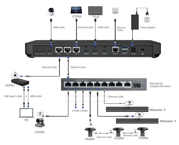
Use the Yealink original power adapter (48V/2A) to charge the endpoint only. The use of the third-party power adapter may cause the damage to the endpoint.
